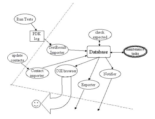
Fig. 3: This figure shows the elements of Pandokia in more detail. The dashed line marks the boundary of the server that hosts the web interface.
